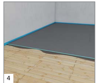
4 Place the building boards onto the adhesive ensuring board joints are staggered.
